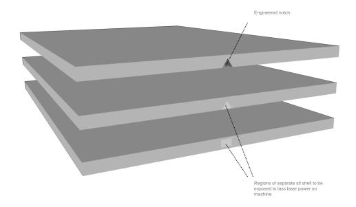
Controlled tear or fracture can be achieved using the traditional approach of physically designing a notch into the geometry.
