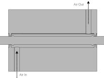
When removing powder rotate and apply pressurized air in tandem to blast the powder out of the axle cavity. Nylon as a natural bearing material will provide a smooth low friction mechanism for low load, low velocity applications. For more demanding applications where friction can generate heat, and wear, consider #3 Inserted Bearings.
