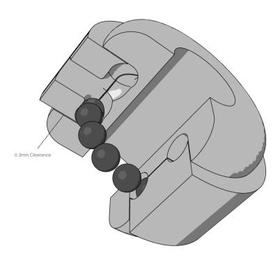
In this example we see the introduction of ceramic ball bearings into a chase, CAD modeled as a torus cavity between the A and B side. It could be considered an integrated hybrid hinge mechanism.
