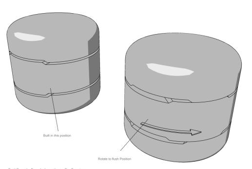
The Balance between functional and quality of mechanism is in play when it comes to the effects of tolerance. Too little clearance and the mechanism will weld together, too much and it will be loose and unreliable.
