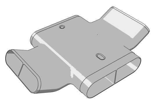
Single elongated connection mount point allows for the thermoplastic variation you see on long sections – Elongate the adaptive Hole at a minimum rate of 5mm per 100mm
