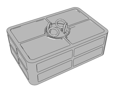
A correctly sintered SLS Nylon Tank (density >0.98g/cc with a wall thickness >1mm is capable of holding both a fluid and a gas under pressure. For Aggressive solvents and Fuels, consider infiltration with Imprex. Often the part cake within the tank, confined by geometry and exposed to extra heat, can become quiet dense and require the application of extra labor for 100% removal.
