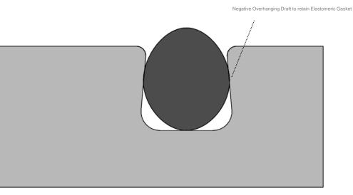
The ability to manufacture "Negative Draft" enables an interesting approach to fixturing of soft elastomeric products like rubber gaskets. You may have to experiment a bit based on the specific durometer of your gasket. Usually a channel with a min width 10% less than that of the uncompressed gasket diameter will both allow both placement and retention of gasket.
