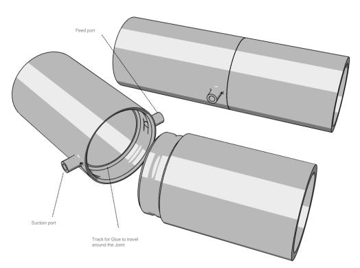
Vacuum draw (not Push) two part thermo set epoxy into the radial channel through the CAD modeled in-out ports at the join intersection to achieve void free sealed coupling. This is a great approach for complex join profiles where you have to guarantee a seal.
