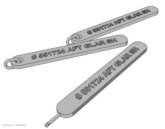
Tags connected by chains or sacrificial sticks are a common way to label SLS parts. Some STL conditioning software packages enable the automatic tagging of parts with STL file name. This is particularly useful in mass custom manufacturing applications. Try to keep all features above 1mm thickness.
