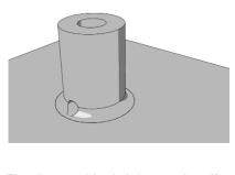
There is no need for draft, however for self tapping plastic screws, its best to apply the principles of conventional design to the surfaces that engage the teeth.
