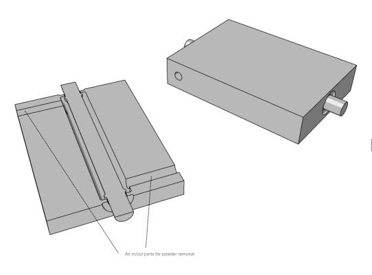
Friction, fit and powder removal are the three factors in play with axle design for SLS manufacturing. Manage friction by applying 1-2mm rails on the static not stressed side of the assembly. Keep the clearance between the rails axle tube at 0.3mm. In regions away from the rails, a clearance of 2mm+ will enable complete and easy powder removal by blowing compressed air through the powder removal access ports modeled into the static side.
