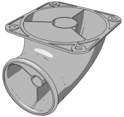
If you need to pass a mounting point through a baffle, elongate and form an aerodynamic teardrop shape to reduce sites for turbulence formation. This will both improve air flow efficiency as well as cut down on noise.
