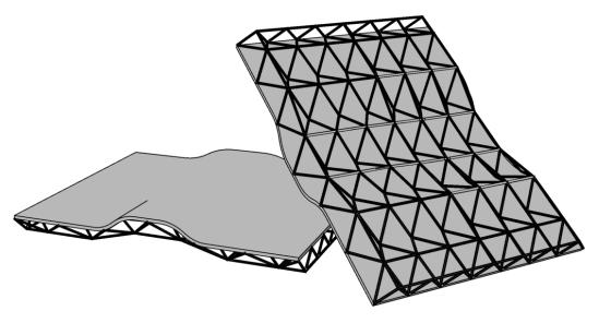
Lattice structures and other designed cellular materials enable designers to put material only where it is needed for a specific application. From a mechanical engineering viewpoint, a key advantage offered by cellular materials is high strength accompanied by a relatively low mass.
