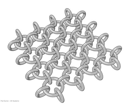
For Basic Chainmail keep the link thickness >0.75mm and the keep clearance between the links over 0.5mm. For large pieces, consider designing the link to have a polygon cross-section in both axis, this will reduce the tremendous file size as well as speeding up the design process.
