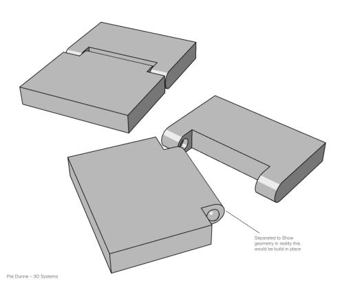
The Sphere in a revolved trapezoidal cone works well for integrated hinges giving good stability, precision, low friction, and high yield. Allow a minimum clearance of 0.2mm between the positive sphere and the pocket.
