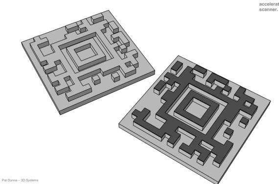
Aztec Barcodes appear to be optimal for SLS Manufacturing. Make the cells <1mm cubed. Note that you must apply contrast ink to the raised surfaces of the barcode to enable or accelerate image capture when exposed to a scanner.
